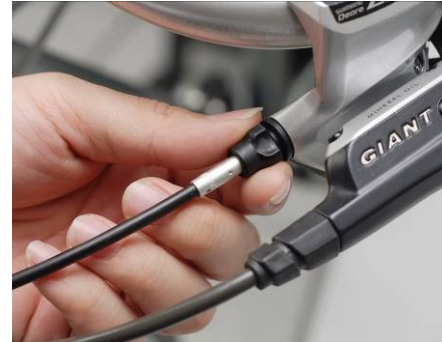
Step 16: Screw the front shifter barrel adjuster completely inward to reserve the adjustment range as much as possible. Check the shifter is at the lowest position possible. Usually #1 on most gear indicators.
