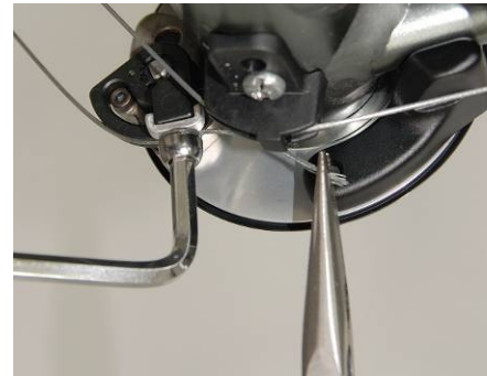
Step 17: Thread the cable down to the cable arm, and install it through the cable pinch plate. Tighten the cable pinch bolt with 5mm hex wrench to a torque value of 50-70 kgf.cm / 5-7 Nm / 45-62 in.lbs.
