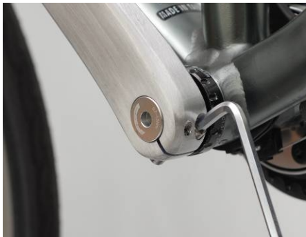
Step 15: Use the 5mm hex wrench "c." to tighten the pinch bolts of the Non-drive side (Left) crank arm ② to a torque value of 110-150 kgf.cm / 10.8-14.7Nm / 96-130 in.lbs.
