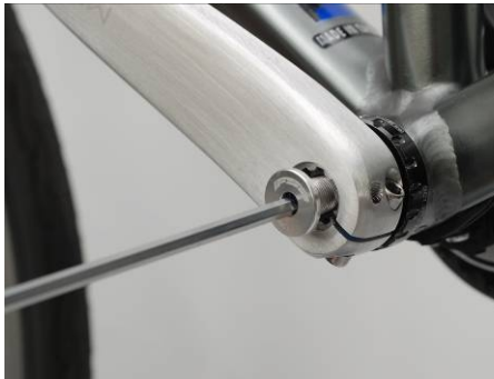
Step 14: Install the Non-drive side (Left) crank arm ② on the BB spindle, ensuring that the crank arms are 180° opposite of each other. Apply medium strength threadlocker to the spindle bolt "B." Use the 5mm hex wrench "c." to tighten the spindle bolt to a torque value of 7-15 kgf.cm / 0.7-1.5 Nm / 6-13 in.lbs.
